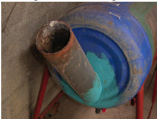
Figure 4 - Inlet of the Digester
