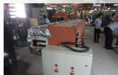
Continuous batch moulding machine developed at the grantee's factory premises
