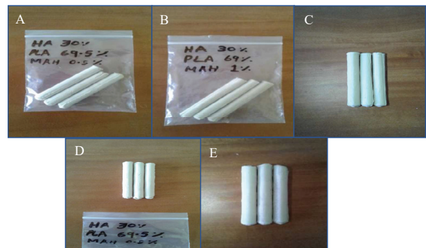
Figure 3: HA/PLA/MAH Biocomposites A) HA30/PLA/0.5MAH; B) HA30/PLA/1MAH; C) HA30/PLA/2MAH; D) HA30/PLA/4MAH; E) HA30/PLA/8MAH
