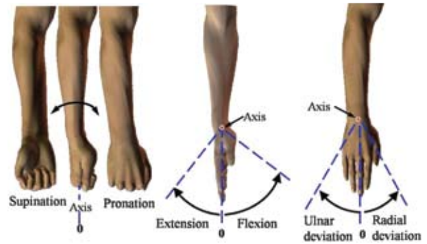
Figure 2: Assisting motions of the W-EXOS. (a) Forearm pronation/supination motion, (b) wrist flexion/extension motion and (c) wrist radial/ulnar deviation
