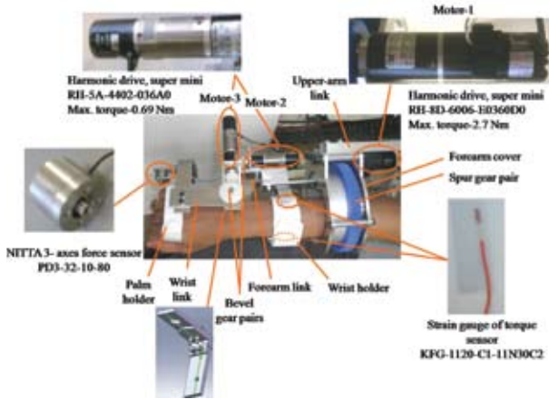
Figure 1: W-EXOS: 3DOF wrist and forearm motion assist exoskeleton robot
