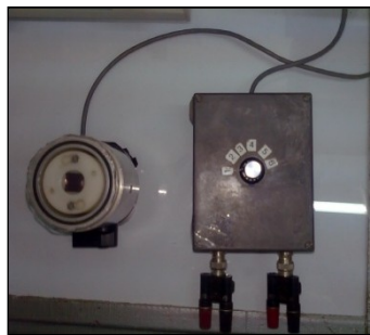
Prepared solar cell in device holder
