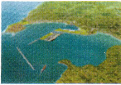
(i) Tsunami breakwaters/ Offshore breakwaters
