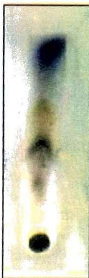
Fig – 7. TLC finger print profile of water extract of Alpinia calcarata rhizome
