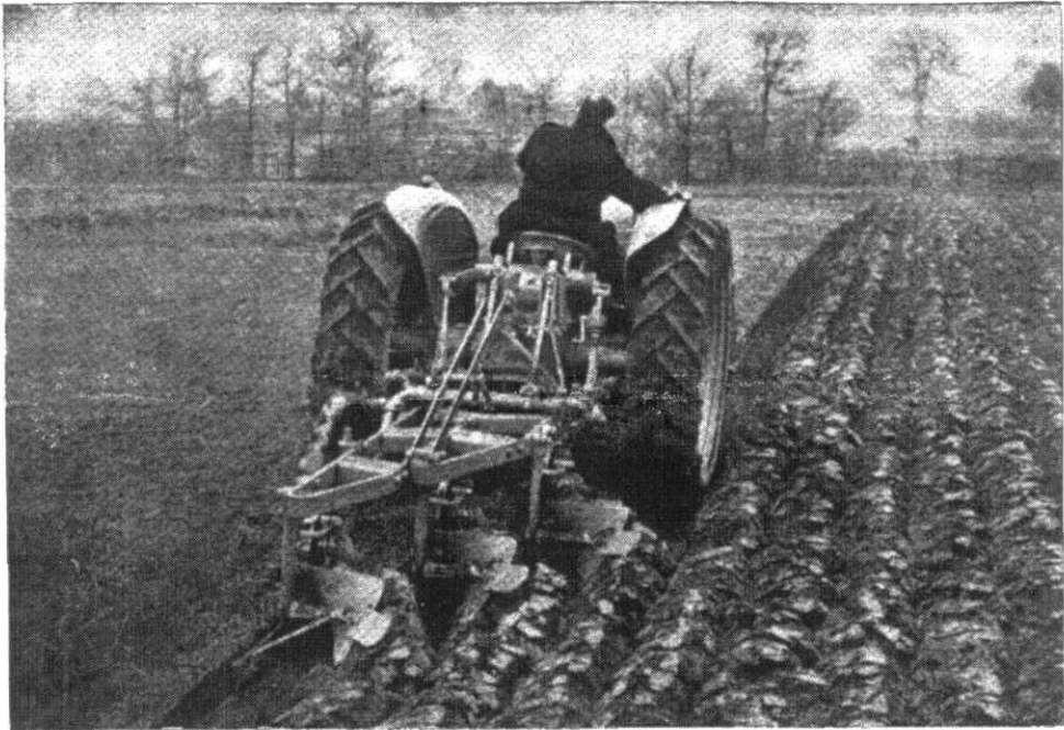
The mechanical plough—a development of the mounted implement which has made small-scale farm mechanisation practicable.
