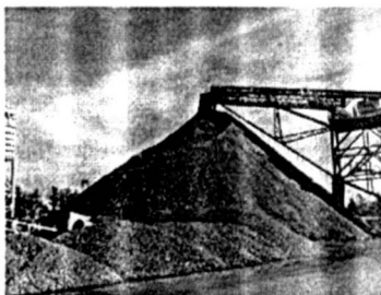
A pile of manufactured sand produced from granite in US
