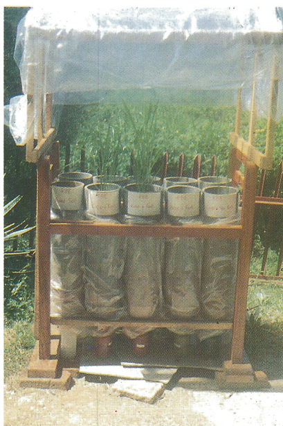
Leaching column experiment to evaluate the changes of K-reserves in an alfisol (CIDA/83/03)
