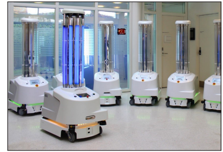
Figure 04 : Ultraviolet disinfection robots
