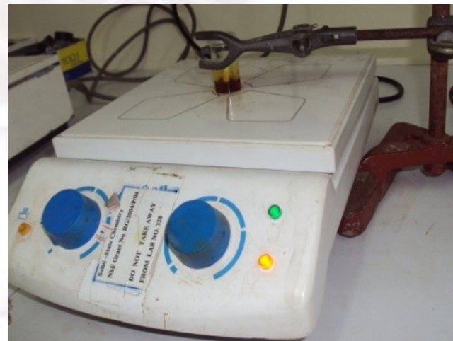
Stirring and heating the composition
