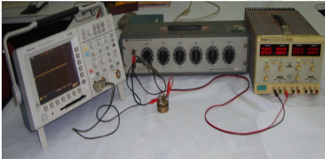
DC polarization set- up
