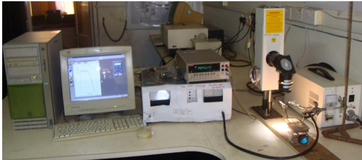
Experimental setup for I-V characterization of DSSC
