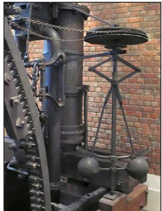
Figure 07 : A Watt Governor on a steam engine at the Science Museum, London
