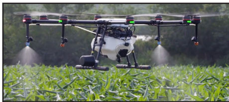
Fig : DJI Agras MG-1S drone spraying over crops
