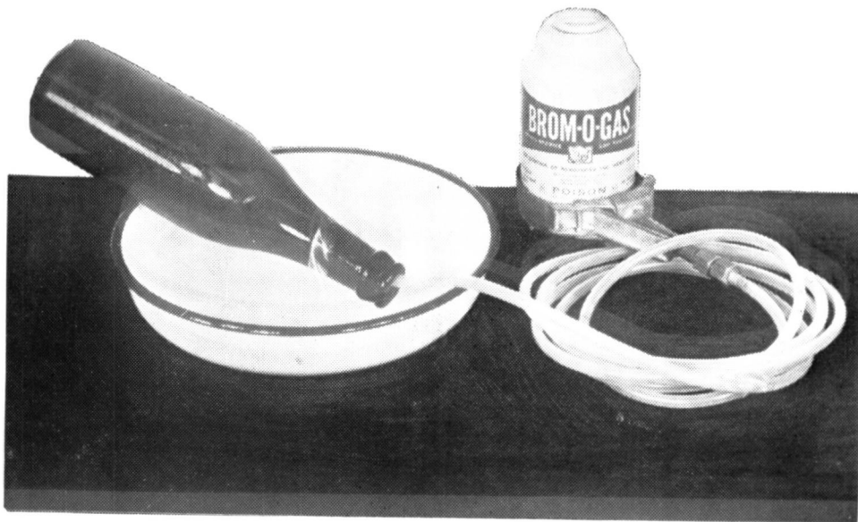
FIGURE 1—Picture shows method of trapping liquid methyl bromide
