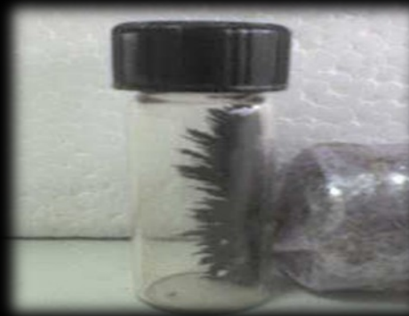
Fig.4 Synthetic set up of magnetic nanoparticles and magnetic attraction
