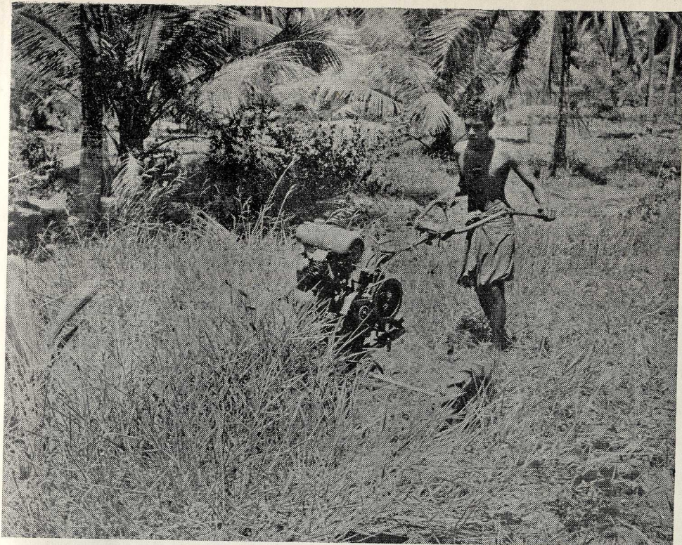
Illustration III — The Landmaster with 36" reciprocating Cutter-bar attachment mows a crop of weeds which have developed in the young plantation.
