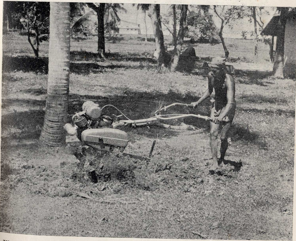
Illustration II — The Landmaster 150 mulching fertilizer round the base of a coconut palm, with its cultivating rotors.
