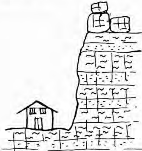
Figure 5.6: Cartoon showing unstable perched block at top of an escarpment. Building below escarpment is in danger from falling block.
