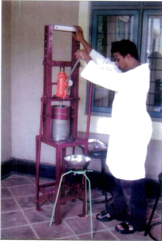
Hydraulic jack operated coconut oil extracting machine
