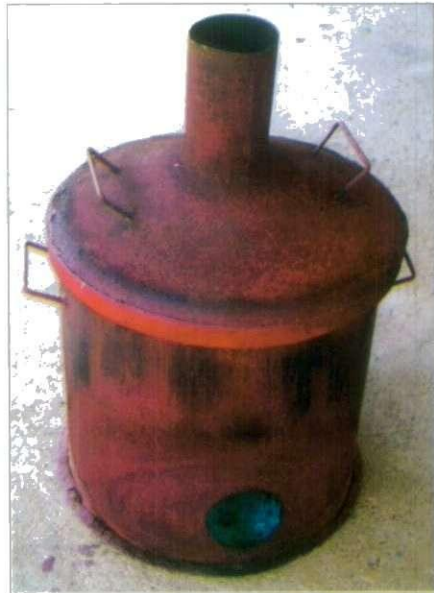
Saw dust burner
